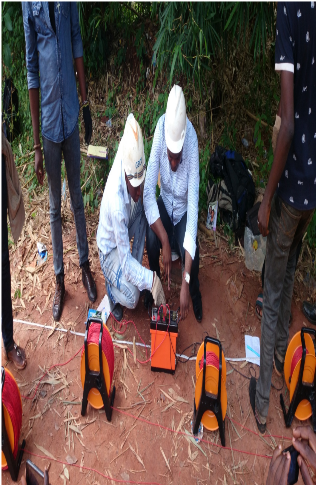
Plate 3.2: Field survey in progress using ABEM Terrameter (Resistivity Meter)
