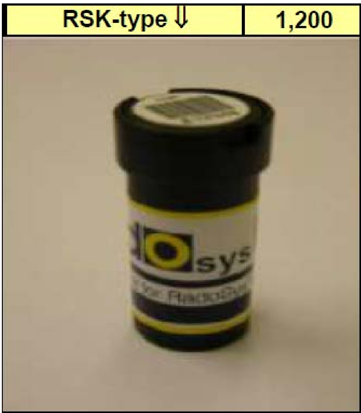
Plate 3.2: Cylindrical exposure chamber (Radopot), 23 mm × 40 mm in dimension
