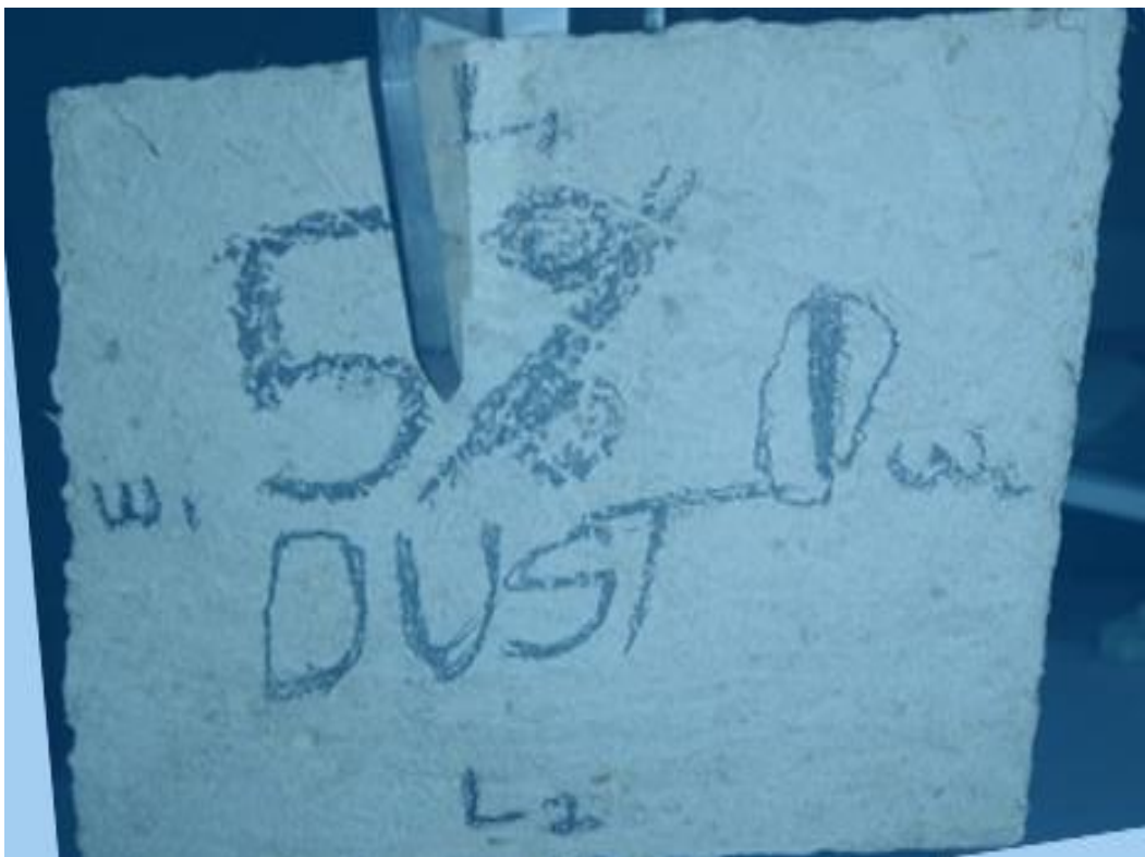
Plate 3.22: Measurement of thickness swelling
