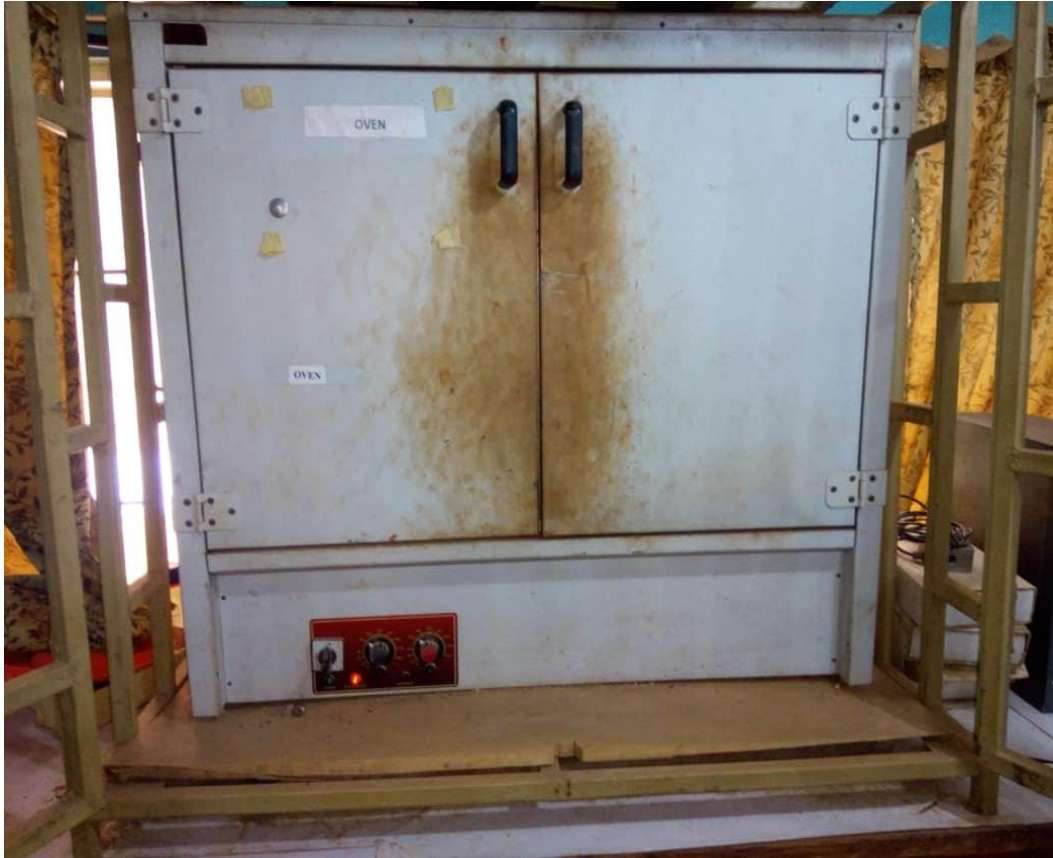
Plate 3.20: Dry oven of composite boards during water absorption test
