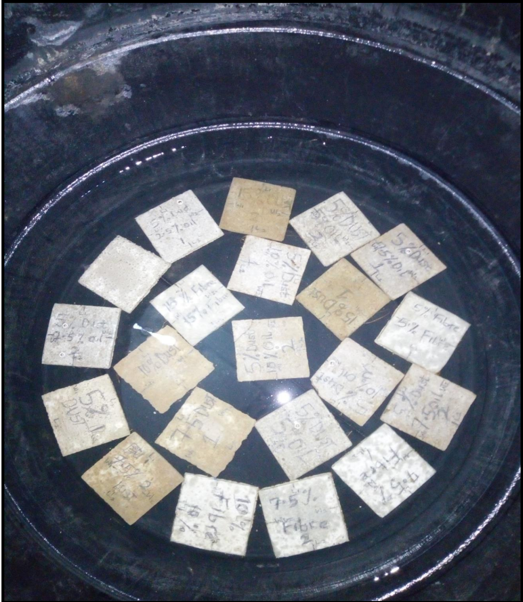
Plate 3.21: Samples immersed in water during water absorption and thickness swelling test
