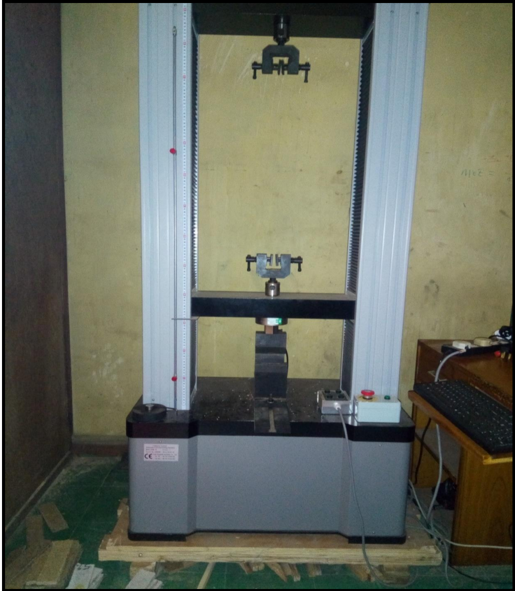
Plate 3.23: Universal Testing Machine for determining MOE and MOR
