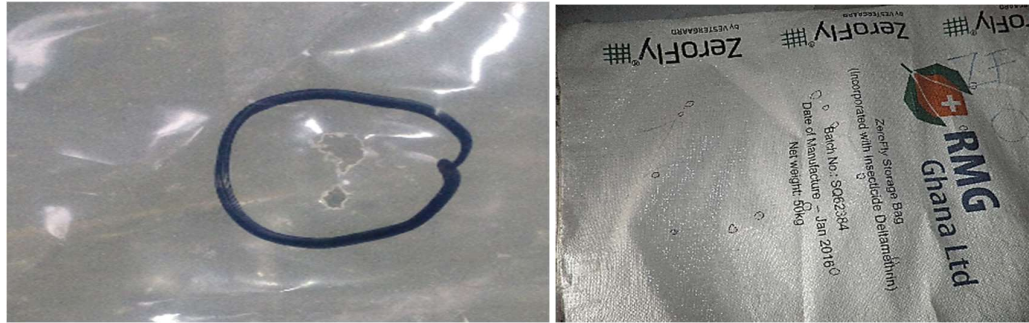
Typical insect exit holes observed on inner HDPE liners and outer woven bags marked with solid circle
