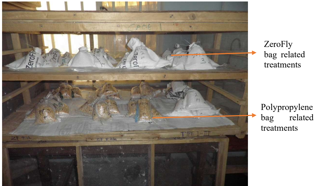
Plate 3.3. Laboratory set up of internally infested P. truncatus and S. zeamais into bagged maize.
