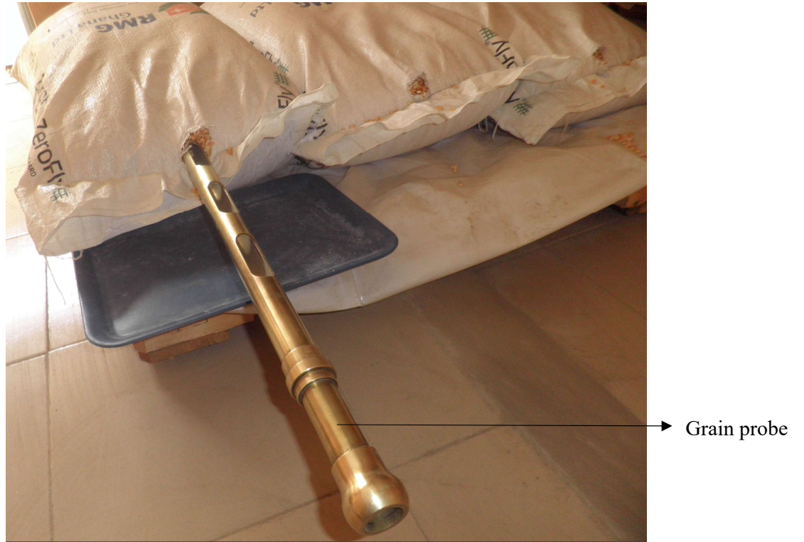
Plate 3.8. Bag opened by cutting to facilitate sampling with grain probe.
