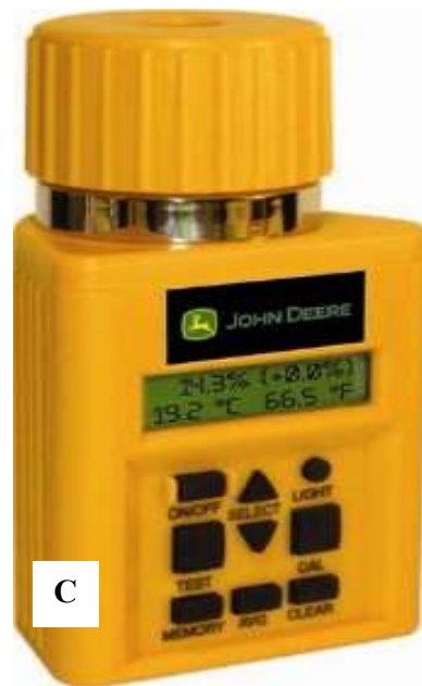
Figure. 3.2. Moisture meters: GrainMate meter (A), Grain Analysis Computer 2100 (B) and John Deere moisture meter (C)
