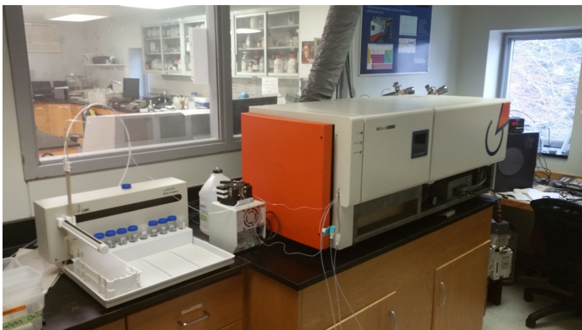
ICP-MS machine used for cations analyses
