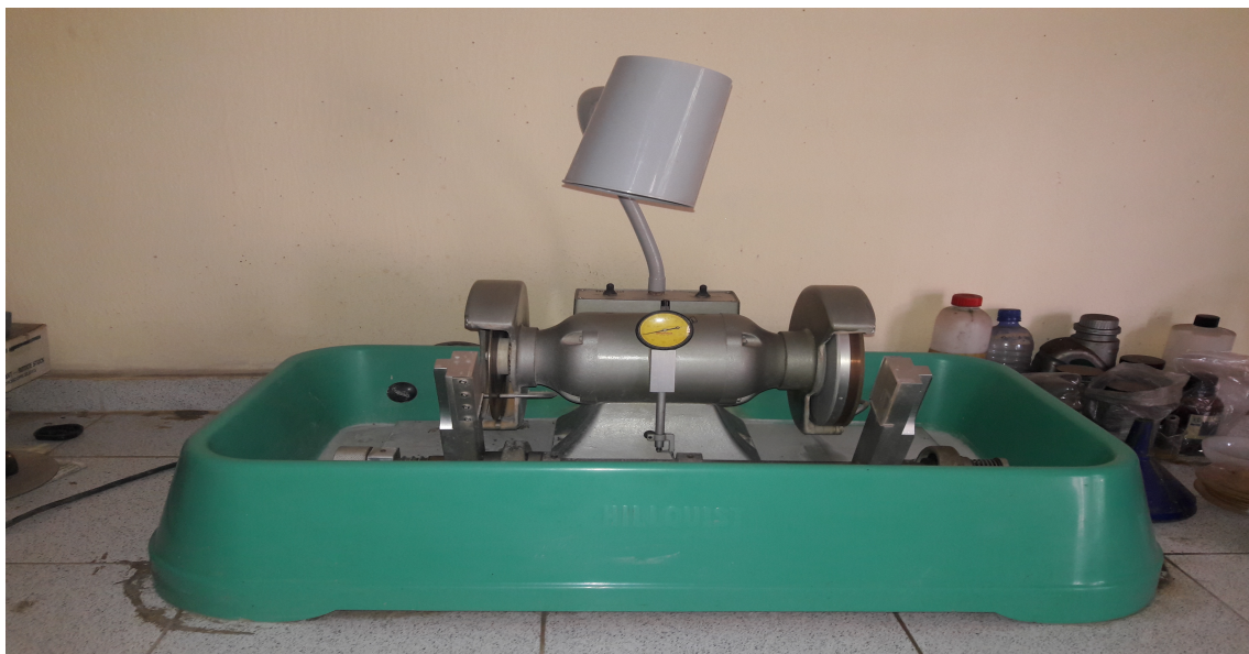
Hillquist Machine for thin section analysis
