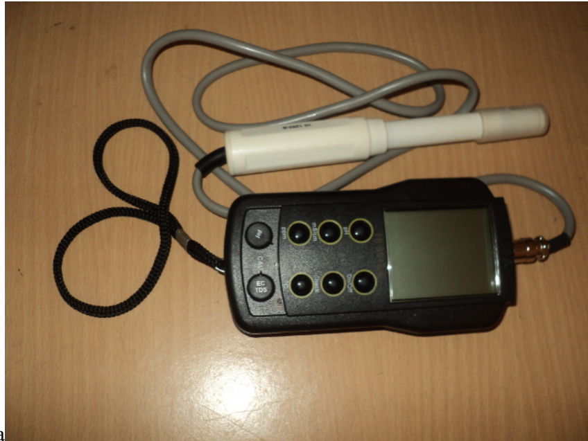
a Conductivity meter used for pH, EC, TDS and Temperature readings
