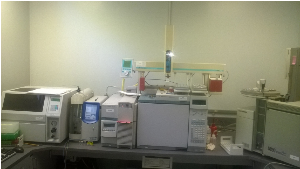
Mass spectrometer used for \delta D analysis
