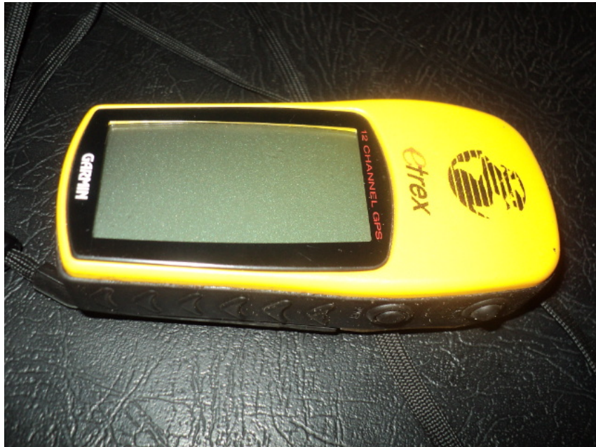
Etrex GPS used for elevation and location readings
