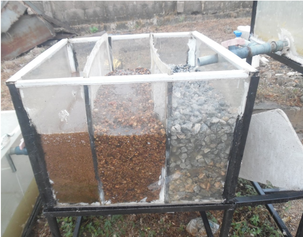
Plate 3.4: The horizontal roughing filter
