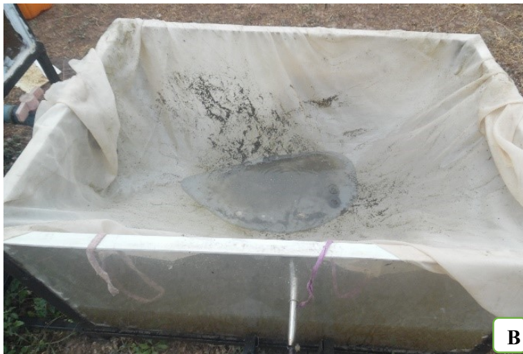
Plate 3.5: Filter cloth used to harvest algae biomass (A - before algae inoculation; B - during harvesting)
