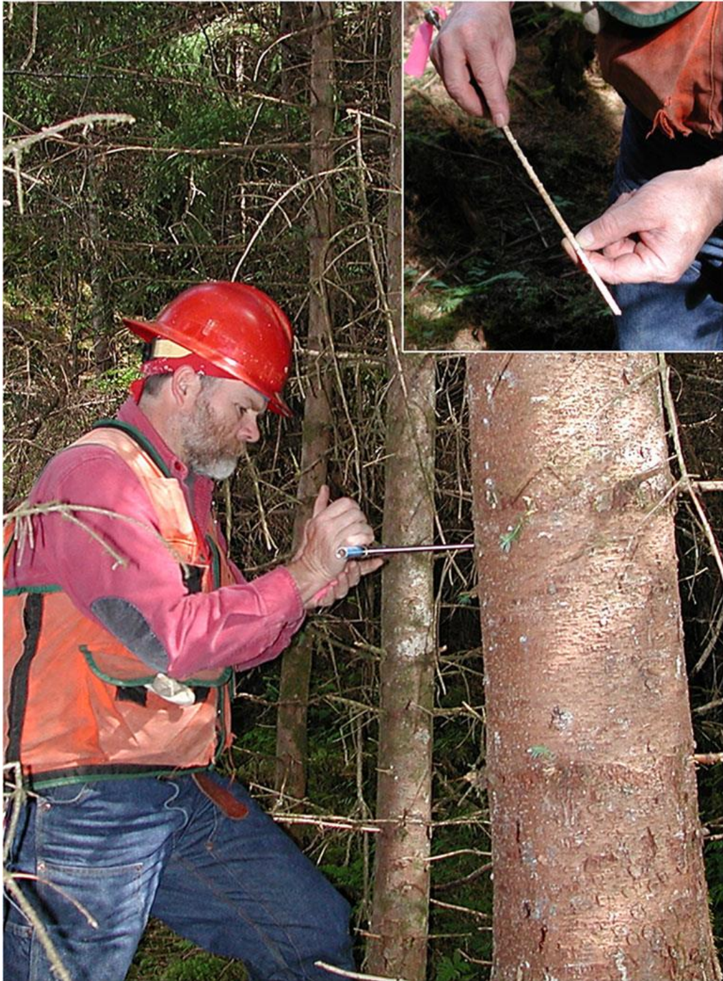
Fig. 2.2. Increment borer being used to extract a core sample from a tree (Gao et al. , 2017)
